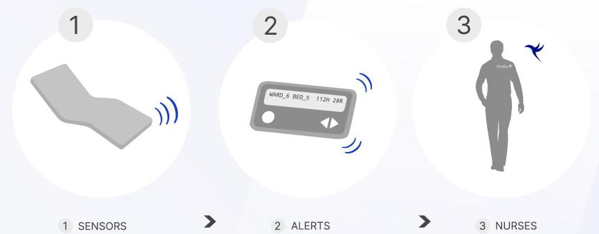
VitalSyn's patented contact-free bed sensor continuously tracks an occupant's average resting heart and respiration rates An alert is sent to the healthcare team whenever rates track outside of safe NEWS2 norms
